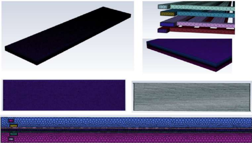
Figure 3: Grid model of the hydrogen fuel cell with parallel reactant flow channels.
